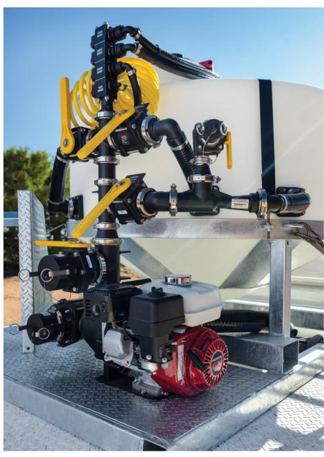
Banjo Venturi Induction system for fast transfer from envirodrums and shuttles
