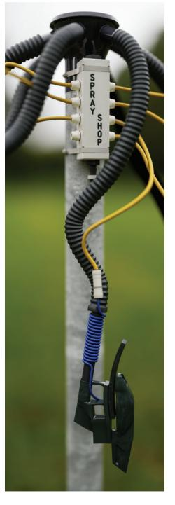
Spray Shop's Liquid Distribution Module 2 is the leading liquid delivery system on the Australian market that has been successfully developed to handle phosphoric acid and offers a 2-year warranty.
